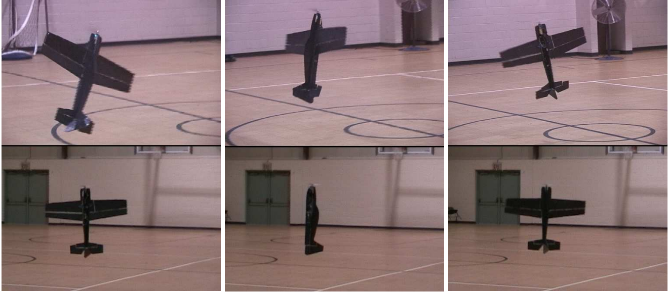
Figure 8: A human pilot hovers a fixed-wing aircraft in a small gymnasium and struggles to keep control (top). Under autonomous control, the same aircraft is able to sustain a hover for more than 90 seconds (bottom).
