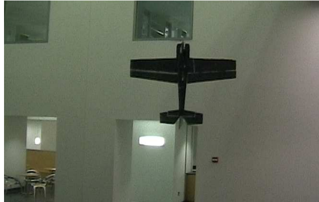
Figure 1: A fixed-wing MAV hovering like a helicopter to stare in a second story window.
