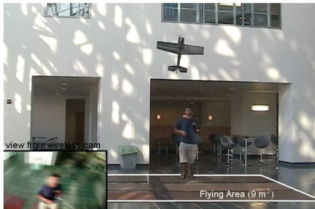
Figure 7: MAV performing a hands-off autonomous hover in and urban structure. Also, a shot from the MAV's bellycam is shown in the bottom left.
