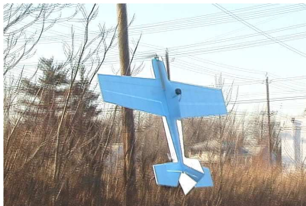
Figure 1: Our MAV prototype combines the endurance of fixed-wing platforms with the hovering capabilities of rotary-wing aircraft. This allows it to carry out missions in cluttered terrain such as forests.
