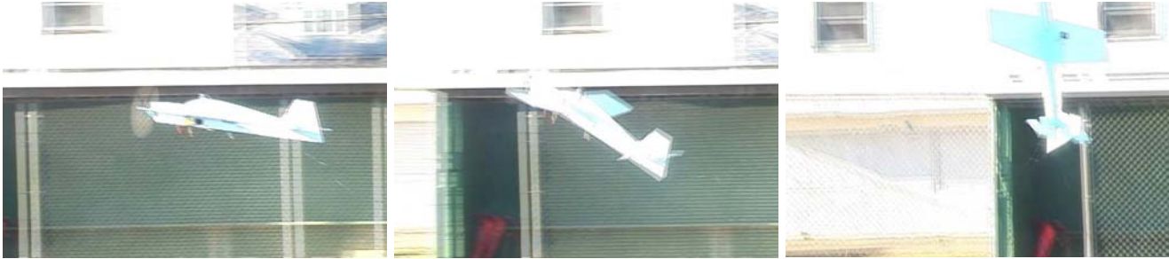
Figure 3: Our MAV prototype with a 30 inch wingspan transitions from cruise flight (left) through the stall regime (middle) and into a hovering position (right).
