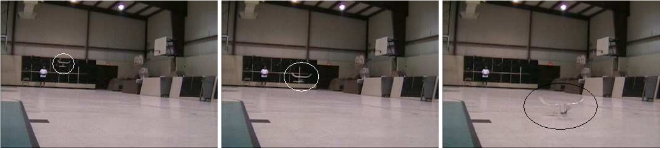
Figure 11: The optic flow on the basketball gym floor is kept constant by the control system. That is, the aircraft (encircled) forward velocity is decreased in proportion with its altitude to land smoothly. Left: Aircraft just after hand launch. Middle: Aircraft midway through landing sequence at proportionally lower altitude and velocity. Right: Aircraft comes to a smooth landing within 25 meters from starting point.
