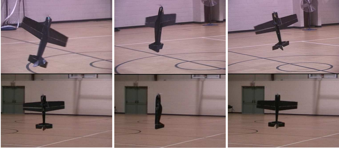
Figure 10: A human pilot hovers a fixed-wing aircraft in a small gymnasium and struggles to sustain a hover (top). Under autonomous control, the same aircraft is able to sustain a hover for more than 90 seconds (bottom).
