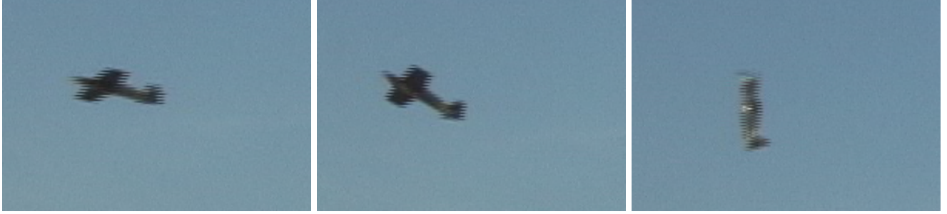
Figure 3: Our MAV prototype with a 90 cm wingspan transitions from cruise flight (left) through the stall regime (middle) and into a hovering position (right) at an altitude of 10 meters (zoomed photos).
