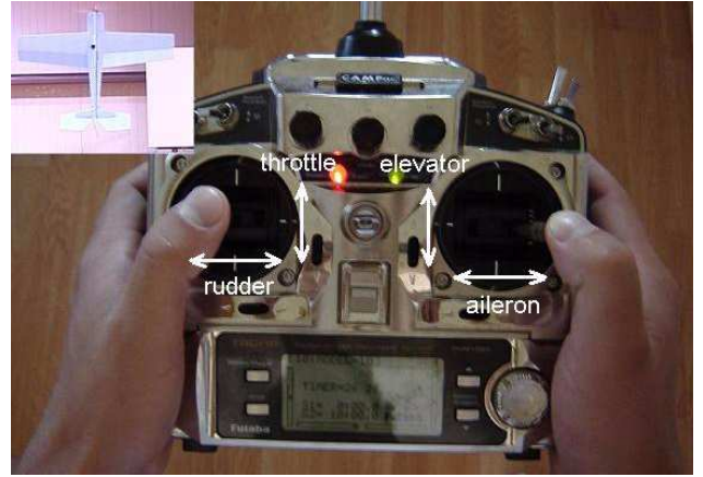
Figure 5: Manual hovering demands control of all four transmitter channels. Inset : simultaneous picture of aircraft in a hover.
