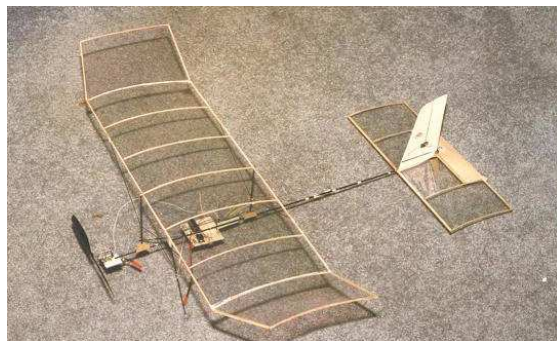
Figure 3: Our 30 gram prototype with 60 cm wingspan flies at speeds of 2 m/s.
