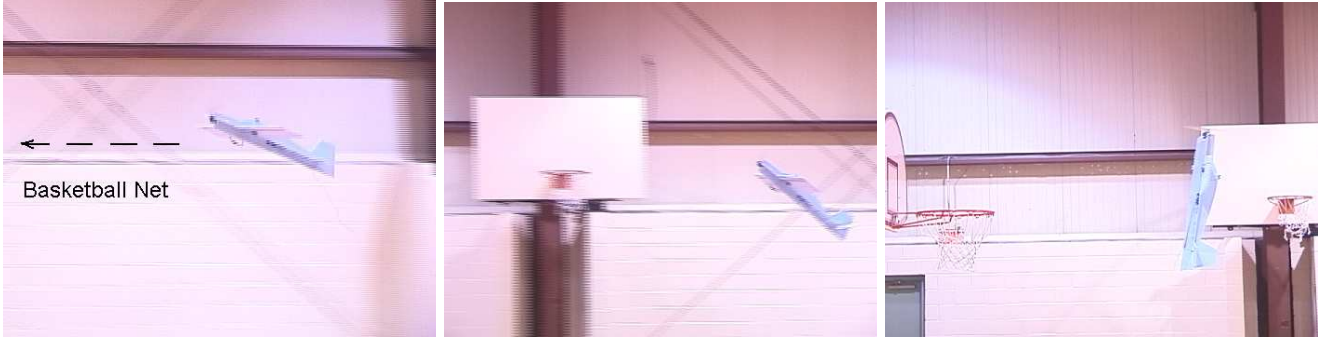
Figure 10: Our MAV prototype with a 1 meter wingspan manually transitions from cruise flight (top left) through the stall regime (top middle) and into a hovering position (top right) to avoid a collision with a basketball net.
