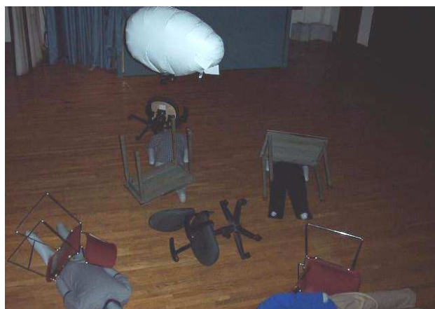
Figure 1: A 30 inch diameter blimp carrying a 14 gram mini wireless camera can provide surveillance images for use in disaster scenarios.
