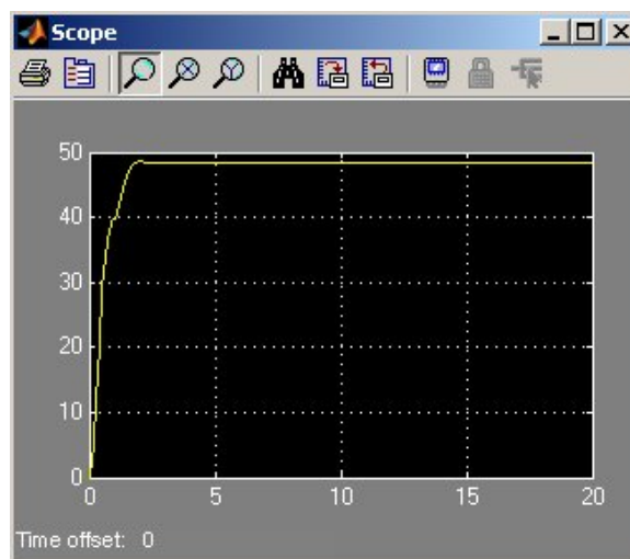
Figure 2: Scope output for PID gains (0.25, 0, 0.5)
