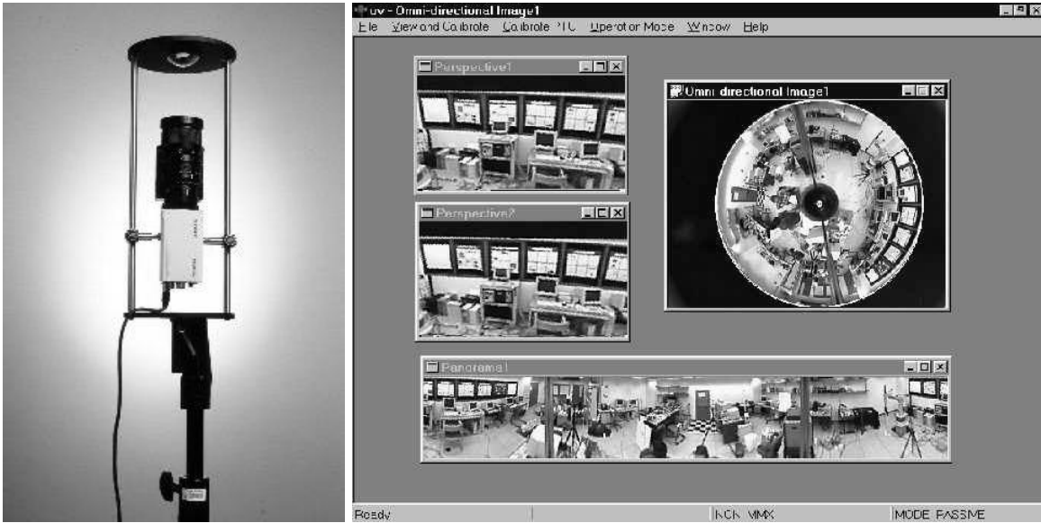
Figure 3: A hemispherical mirror mounted in front of a camera lens (left) can capture 180° fields-of-view (right circular image). Un-warping the image provides a set of conventional 2-dimensional images
